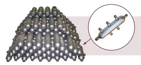
Condensate and seal pots are used as a barrier between the main line and the secondary instruments in the flow and pressure measurement of liquids, steam, or other vapours that can affect secondary instruments.
