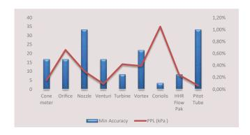
Venturi tubes and HHR flow tubes provide the highest level of traceable accuracy with minimal pressure loss. The main advantage of the FloTec pitot tubes lies in an even lower pressure drop (<10 % of the differential pressure) as well as in the constant measurement accuracy over a wide range of Reynolds numbers.
