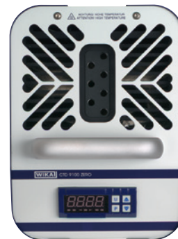
Fig. 2: Temperature block with seven test bores
