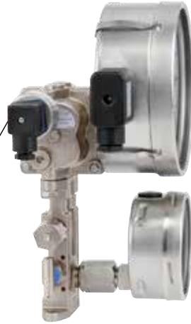
The transmitter for the working pressure is mounted to the minus side of the DP cell and can be installed on site.
