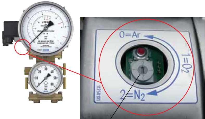
BCD switch (scale selection switch) and zero point key (sealing cap removed)
