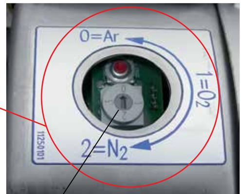
BCD switch (scale selection switch) and zero point key (sealing cap removed)
