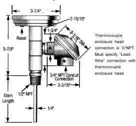
Type TT.30 w/thermocouple connection
