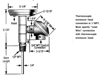
Type TT.50 w/thermocouple connection
