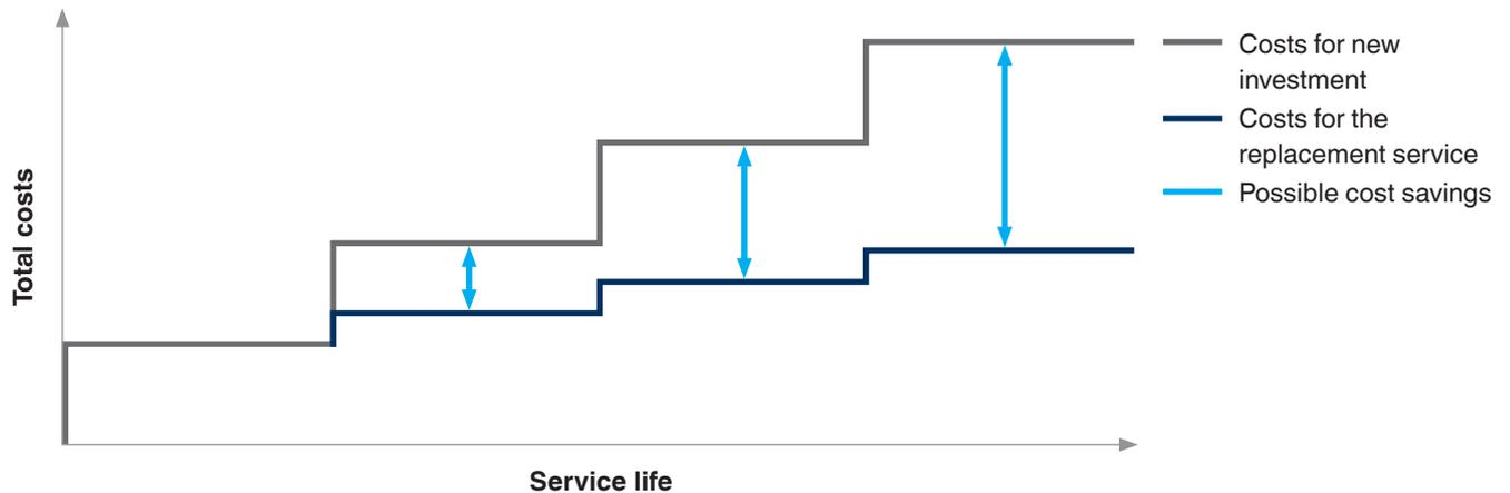
With the replacement service, the total costs of the diaphragm seal system can be clearly lowered. In this way, the service life of the process transmitters can be fully utilised
