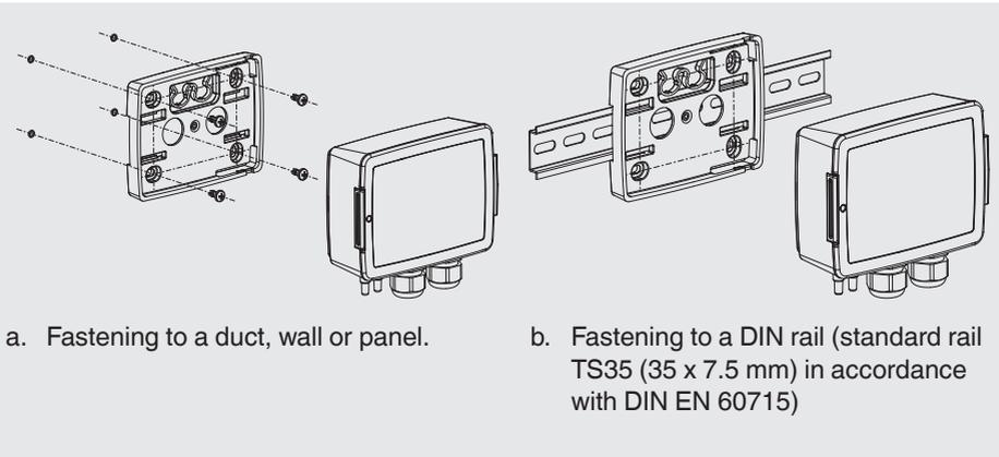
a. Fastening to a duct, wall or panel.
