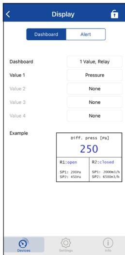
The colour change of the set limit values can be defined under “Alarm”. The displayed value can take on up to three different colours. E.g., in the case of a supply air filter, the normal value can be displayed in WIKA blue, the pre-alarm in yellow and the alarm in red. The colours can be freely-selected using RGB.
