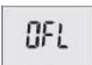
This indicates that the applied pressure is outside of the full scale range. If the message will remain displayed while the CPG500 is pressure less, please contact WIKA.
