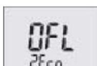
**OFL/Zero** is displayed for 3 seconds if the measured pressure (0 bar) is greater than 5% of the measurement range.
