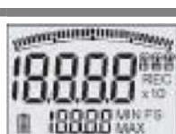
A self-test procedure is carried out
