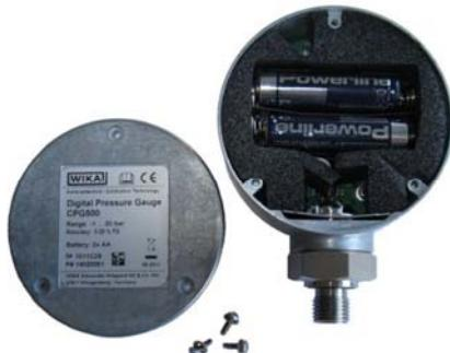
Open the battery compartment. Insert the new batteries as depicted.
